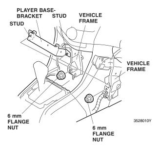
Insert the studs of the left and right player subbrackets into the holes in the vehicle frame, then install one 6 mm flange nut on the end of each stud while pushing each subbracket upward.
