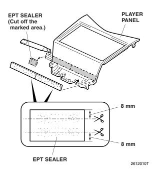
23. Clean the player panel with isopropyl alcohol where the EPT sealers will attach. Attach the EPT sealer to the player panel and cut off the marked area from the player panel.
