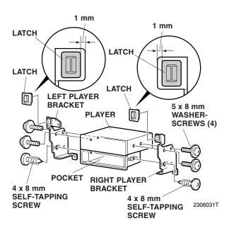
12. Position the left and right player brackets on the player and pocket, and install four 5 x 8 mm washer-screws, and two 4 x 8 mm self-tapping screws.
