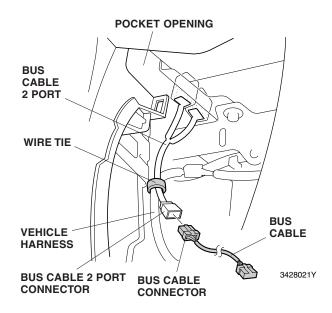
17. Secure the BUS cable 2 port to the vehicle harness with the one wire tie.
