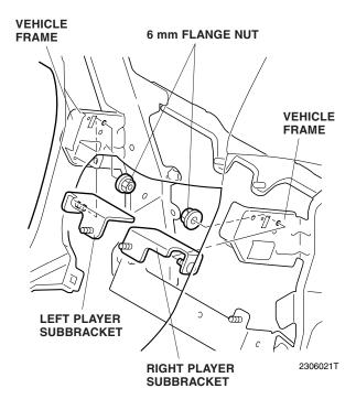
If you are installing an in-dash CD player, remove the shipping bracket.
